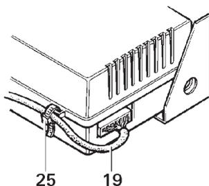
For strain relief, secure control panel cable (19) on the control electronics by means of enclosed cleat (25).
