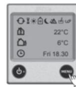
Launch the settings menu by pressing the MENU button. The background light comes on and those functions that can be set are displayed. Settings that you make are automatically saved after 10 seconds.
