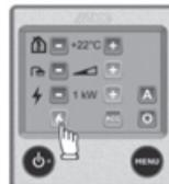
Start gas operation by pressing the LPG flame symbol. The LPG symbol is activated and changes colour to green.
