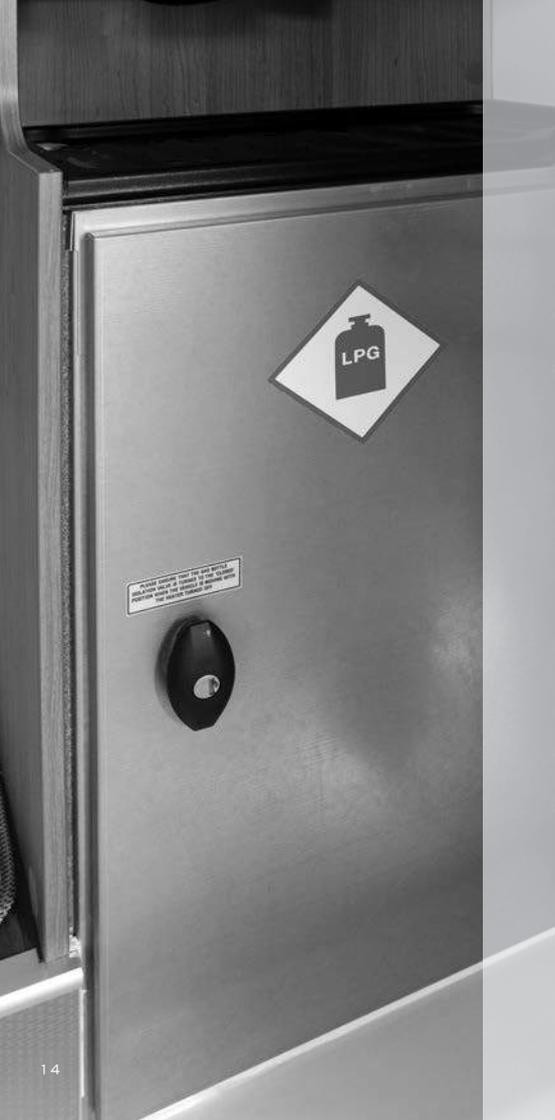
The gas appliances in your vehicle are fed from a gas cylinder that is housed in a sealed cylinder compartment or an underslung fixed LPG tank.
