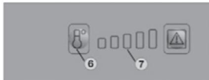
Select the desired cooling compartment temperature by pressing button (6). The LED display (7) of the selected temperature is illuminated.
