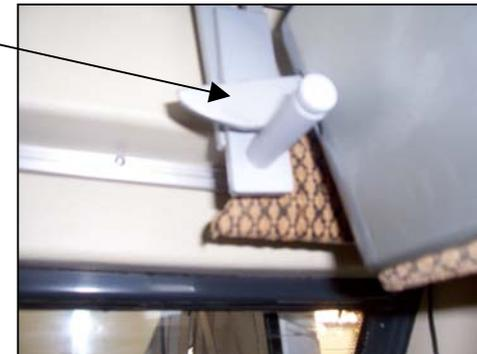
Ensure locking bars are fully latched over the locking pins
