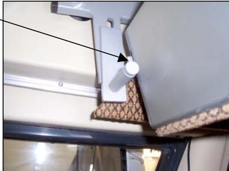
When the locking handle is pulled forwards the locking bars retract over the locking pins and the bed can be pulled down for use
