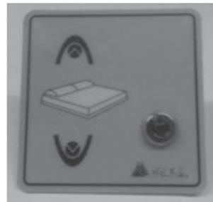
The bed is operated from a small aluminium panel with security key and two buttons. The upper button will move the bed upwards, the lower button will move the bed downwards.
