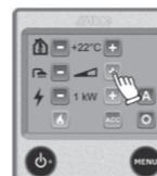
If there is freshwater in the heater and hot water is required, press the + button (the symbol will then show half-shaded). Press the - button to reduce the water temperature.
