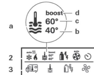
a = Boiler \* – Warm water boiler is switched on.
