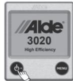
To start the boiler, press the on/off button and the start-up display appears. The boiler starts with the last selected settings. A green LED comes on beside the on/off button when the panel/heating system is on.
