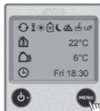
Launch the settings menu by pressing the MENU button. The background light comes on and those functions that can be set are displayed. Settings that you make are automatically saved after 10 seconds.
