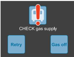
Make sure there is gas in the bottle, no blockage in the gas line. At temperatures below 5°C use the Propane rather than Butane.
