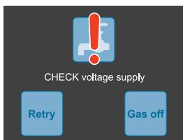
Ensure voltage is above 12V and below 15V. This can be done by recharging the battery.
