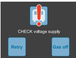
Ensure voltage is above 12V and below 15V. This can be done by recharging the battery.
