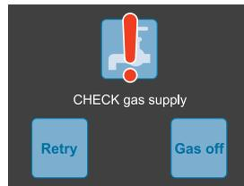
Make sure there is gas in the bottle, no blockage in the gas line. At temperatures below 5°C use Propane rather than Butane.
