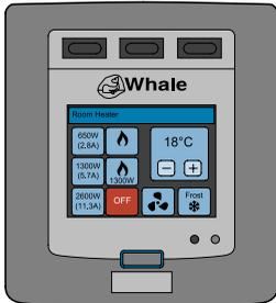
Fig 3 Space Heater Functions
