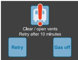
The heater has overheated due to the vents being either closed or blocked, for example with a cushion or a bag. Remove the blockage and open any closed vents. Leave the heater for 10 minutes to cool down, then try again.
