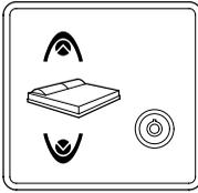
The bed is operated from a small aluminium panel with security key and two buttons, one to move the plane of the bed upwards, the other downwards.
