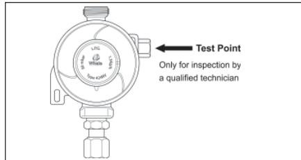
Your new motorhome has been fitted with a fully approved gas regulator designed to operate with both Butane and Propane gas at a gas pressure of 30mBar. Your regulator is fitted with a test point, which is accessed via the inlet at the side of the regulator. This access point is only for carrying out gas pressure tests and **must not** be used for any other purpose.
