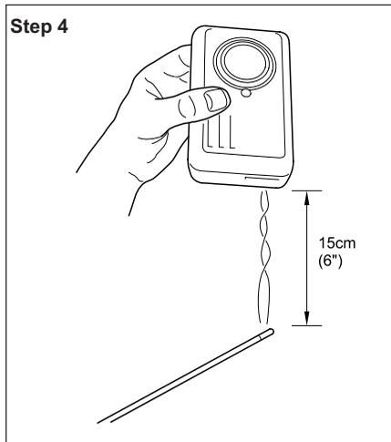
Turn the detector on its side so that the vents on the right hand side of the detector are pointing downwards. Hold the burning incense stick around 15cm (6 inches) below the detector, so that the smoke enters the vents on the side of the detector. An increase in the localised carbon monoxide level within the sensor to more than 50ppm will cause the sounder to sound for one cycle of
