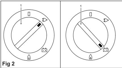
Switch on the appliance by turning the energy selection switch (1) clockwise to position:
