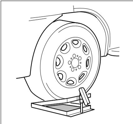
Place the leveller jack, folded flat, in front of the wheel that is to be raised to level the axle. Drive the motorhome onto the leveler jack and adjust the height until the spirit level shows that the motorhome is laterally level.
