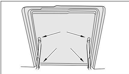
For easier cleaning, the dome can be removed from the inner frame by releasing the four plastic split pins.
