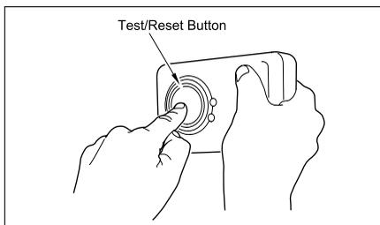
Cover the sounder vents with one hand. Press and hold the Test/Reset button down with your thumb/finger until the Power LED illuminates green and the sounder sounds for a second time (this should happen after around 5 seconds). Release the Test/Reset button. Upon releasing the Test/Reset button the Power LED will flash green once every second. This indicates that the sampling rate of the detector has increased and can be tested using a known source of CO.
