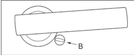
To open and close the door, push the lever down.
