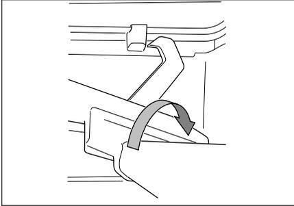
To open the rooflight, both pleated blinds must be open.
