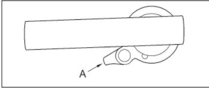
To lock the door, push the small lever down (identified in the drawing as A) then to unlock, push this lever back to the original position.
