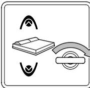
Insert the key into the lock and turn clockwise 90°. Press the top button to bring up the bed. The bed moves as long as the button is pressed to lift.
