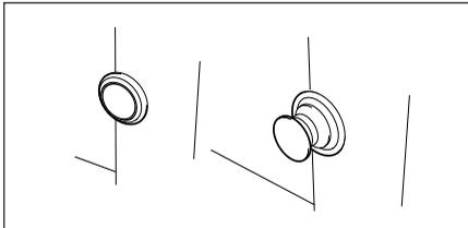
Other internal doors such as the wardrobe and table storage locker are fitted with a 2-position button lock. Push the button to lock the door and the button should remain flush with the door. Push the button again to release and the button should then protrude from the door surface.
