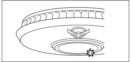
**Note:** The test button accurately tests the alarm's smoke sensing circuit, there is no need to test your alarm with smoke. If your smoke alarm fails to give an audible test signal, please refer immediately to the trouble shooting guide at the end of this manual.
