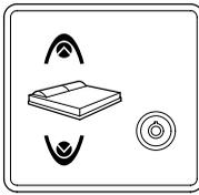
The bed is operated from a small aluminium panel with security key and two buttons, one to move the plane of the bed upwards, the other downwards.
