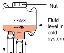
Fig. 11 Expansion Vessel
