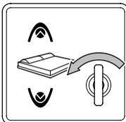
Once the bed reaches the desired position, turn the key to the OFF position, turning it to the left by 90°.
