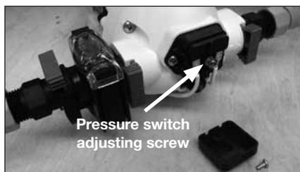
The pump may have to be removed to gain access to the adjusting screw. Drain the water system before removing the pump.
