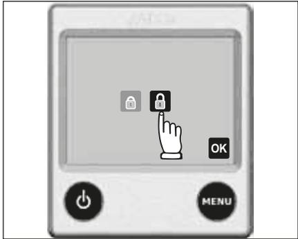
2. The control panel in unlocking menu. Press on open padlock, then OK or MENU to unlock the tools menu. When activated the symbol changes colour to green.
