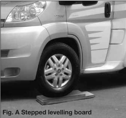
**Fig. A Stepped levelling board**
