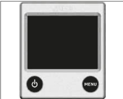
2. To start the boiler, press the On/Off button and the start-up display is displayed. The boiler starts with the last selected setting.
