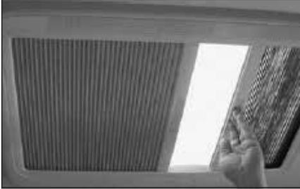
The blind and flyscreen operate independently of each other and are engaged by connecting to each other and sliding.
