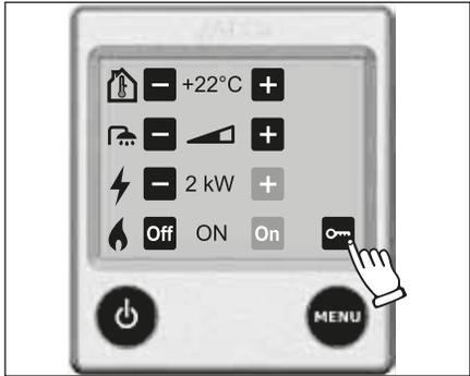
1. The control panel in setting menu. Press the unlock symbol.
