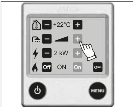
1. Increase the quantity of warm water by pressing the + button. When activated the plus symbol changes colour to green.
