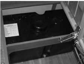
**Escape fresh water tank showing central cleaning hatch**
