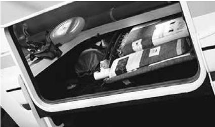
Some models are provided with exterior access locker doors. These are suitable for storing external equipment.
