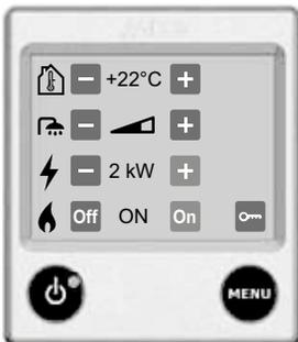
**Note:** if “Standby Brightness” is set to Off, the display goes out when it enters standby mode, but lights up if you press the screen. See settings under 9.12.
