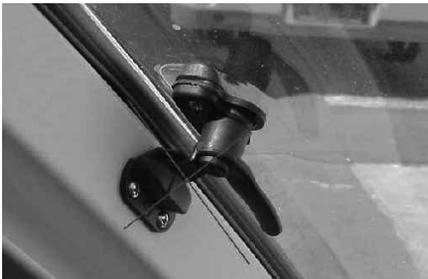
To close, turn the handle clockwise until the dome lies on the seal and a resistance is noticeable.
