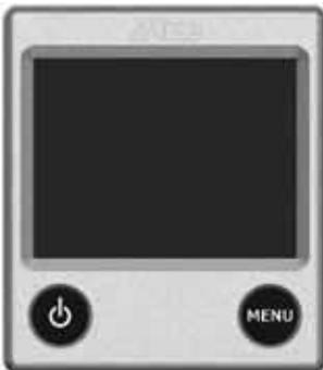
2. To start the boiler, press the On/Off button and the start-up display is displayed. The boiler starts with the last selected setting.
