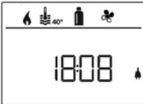
If no entry is made within a few minutes, the standby screen is automatically shown again. The display shows the time and current room temperature alternately.
