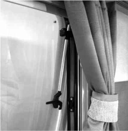
To open, turn knobs anti-clockwise and open catches. Swivel the window pane open to the desired position and close knobs clockwise to lock in the open position.
