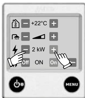
1. Start and step between the various power steps (Off, 1kW, 2kW or 3kW) with the + button or – button. The set value is displayed on the screen. When activated the plus symbol changes colour to green. (Certain boilers are equipped with max 2 kW, selecting 3kW is not possible in these cases.)
