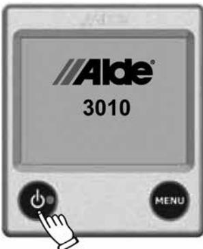
A green LED comes on beside the On-/Off button when the panel/boiler is on.
