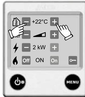
1. The temperature displayed is the temperature which is set at present (in this case 22.0°C).
