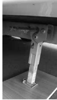
**Fig. A Winding the corner steady**
