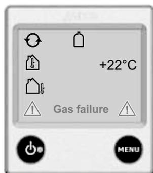
If an error occurs in the system, the display will show the reason. This is only displayed when the panel is on standby.
