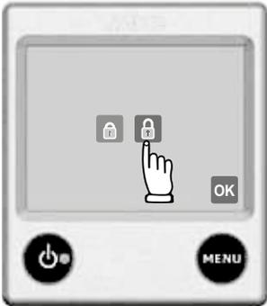
3. The control panel in setting menu with unlocked tool menu. In order to get to the tool menu, press the symbol.
