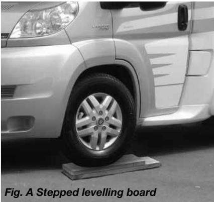
**Fig. A Stepped levelling board**
