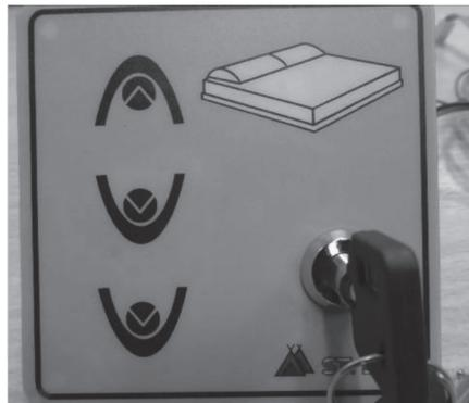
Once the bed reaches the desired position, turn the key to the OFF position, turning it to the left by 90° and remove it.
