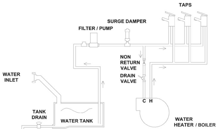
When power is supplied to the pump, it will draw water from the water tank, and pump it to the motorhome taps, shower and water heater.
