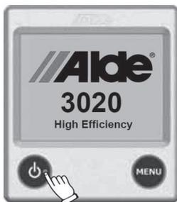
The system will now be drawing variable 0.1–1.5 A of current from the 12v supply.
