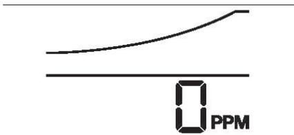
FireAngel's unique digital read out displays the amount of CO that the sensor is detecting shown in parts per million (PPM). It is designed to indicate levels from 10PPM to 999PPM.
