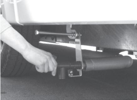
Once the tank has drained, close the valve and rotate the bracket anti-clockwise (if on the nearside and clockwise if on the offside) to return it to the 'stowed' position.
