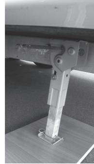
**Fig. A Winding the corner steady**
