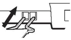
**Note:** If the disabling tab is no longer available then the clip can be replicated by opening out a thin metal paper clip into a U-shape.
