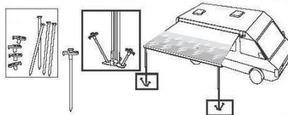
If you want to fasten the support legs to the vehicle, put the terminals into the wall brackets. The brackets can be fixed only in reinforced points.
