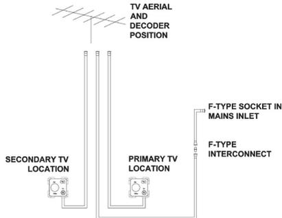
A short co-ax lead featuring a screw on co-ax connection will be present behind the Blue mains inlet connector. A co-ax cable will be fitted and connected within the motorhome, from the back of this connection, to the location intended for the later fitment of a satellite decoder or similar receiver.
