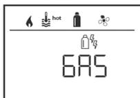
**Note:** The select energy type menu is displayed if a heating system with electric heating elements is connected.
