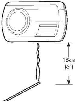
**Note:** We suggest the use of an incense stick or cigarette as the way in which these products burn produces a readable localised amount of CO. A readable level of carbon monoxide will not be given off by other sources of smoke, for example an extinguished candle or match.
