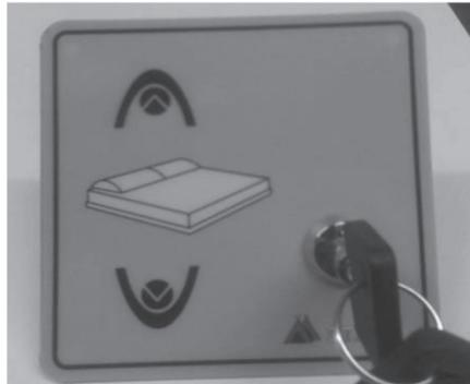
Once the bed reaches the desired position, turn the key to the OFF position, turning it to the left by 90° and remove it.
