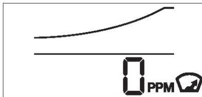
**Note:** It is possible and quite normal for the peak level to remain at 0ppm, i.e. this simply means that the alarm has not detected any CO in the last 4 weeks.
