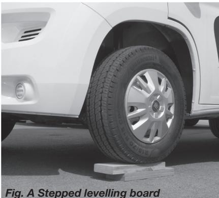
**Fig. A Stepped levelling board**
