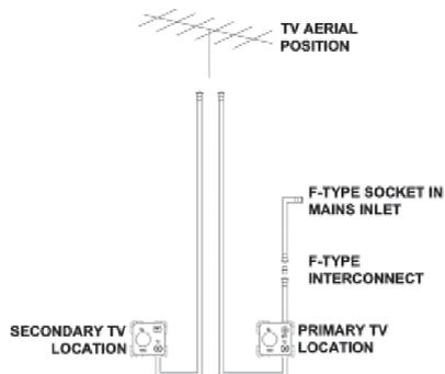
A short co-ax lead featuring a screw on co-ax connection will be present behind the Blue mains inlet connector. A co-ax cable will be fitted and connected within the motorhome, from the back of this connection, to the primary TV position within the motorhome. At the same time, further co-ax cable or cables will be fitted which route from the TV aerial position (i.e. within the wardrobe) to each of the TV positions within the motorhomes.
