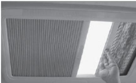
The blind and flyscreen operate independently of each other and are engaged by connecting to each other and sliding.
