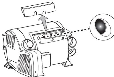
To reset the overheating protection, allow heater to cool, remove connection cover and press red reset button.
