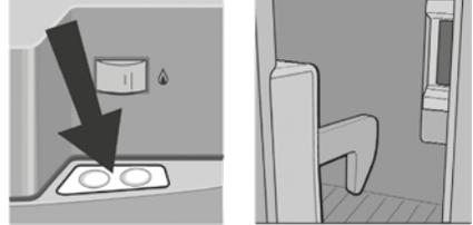
Open the door by pressing the locking button and pull open. Shut the door again by pushing it to close. The snapping into the lock can be heard. While the vehicle is parked, the locking hook may be fixed to facilitate opening of the door.
