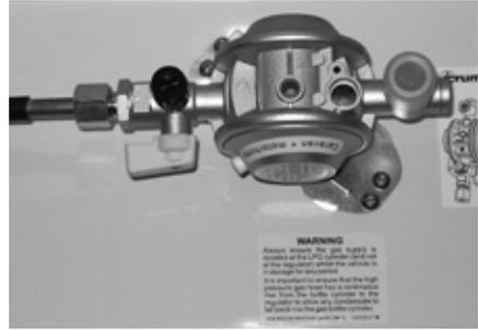
Your motorhome is supplied with a wall mounted gas regulator plumbed inside the gas cylinder compartment. The regulator and all appliances work at a harmonised 30mb pressure, which work with Butane and Propane gas.
