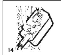
5. Slide the holding tank into position through access door (fig. 5).
