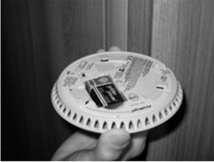
3. Replace the alarm on its mounting plate, lining up the large central vent on the front of the alarm, with the 'X' that is moulded into the plastic on the mounting plate (if unsure see page 13 of the alarm user manual). Ensure the unit is securely fitted.
