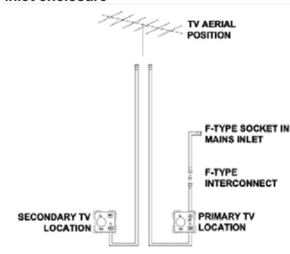
A short co-ax lead featuring a screw on co-ax connection will be present behind the Blue mains inlet connector. A co-ax cable will be fitted and connected within the motorhome, from the back of this connection, to the primary TV position within the motorhome.
