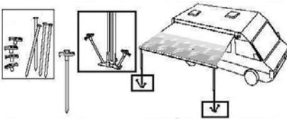
If you want to fasten the support legs to the vehicle, put the terminals into the wall brackets. The brackets can be fixed only in reinforced points.
