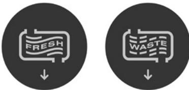
**Fresh and Waste tank drain switch**
