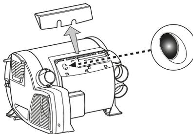
To reset the overheating protection, allow heater to cool, remove connection cover and press red reset button.
