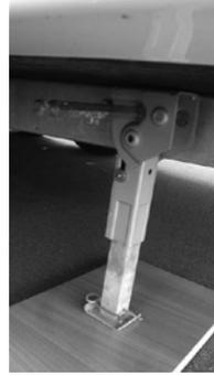
**Fig. A Winding the corner steady**
