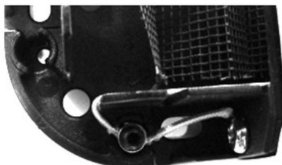
In each corner piece there is an cord tensioner (see photo). By unscrewing the hexagon screw, the cord can move through the cord tensioner. When you pull the cord, the tension will get higher, when you let it move back the tension will get less.
