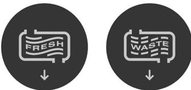
**Fresh and Waste tank drain switch**
