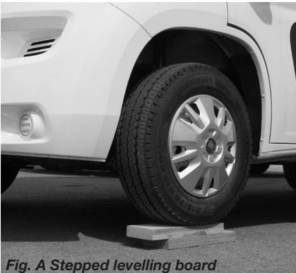
**Fig. A Stepped levelling board**
