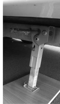
**Fig. A Winding the corner steady**
