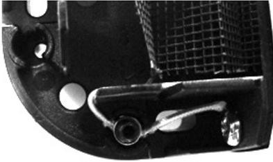
In each corner piece there is an cord tensioner (see photo). By unscrewing the hexagon screw, the cord can move through the cord tensioner. When you pull the cord, the tension will get higher, when you let it move back the tension will get less.
