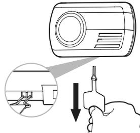
Your motorhome is fitted with a Fireangel CO-9D Carbon Monoxide Alarm. To activate the alarm pull the disabling tab as shown in the above image. Please read the instructions for the alarm, which are available at the following location:
