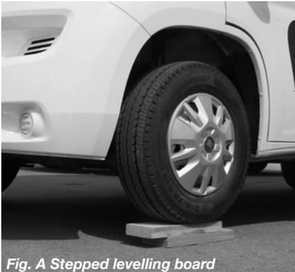
*Fig. A Stepped levelling board*
