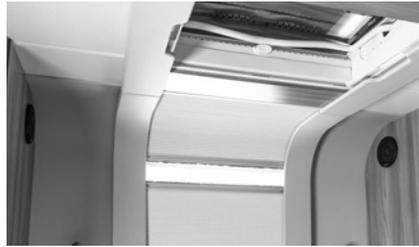
The blind and flyscreen operate independently of each other and are engaged by connecting to each other and sliding.
