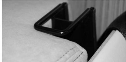
Top tether anchor points are fitted on the upper seatbelt stanchion and are accessed by removing an insert on the backrest cushion.
