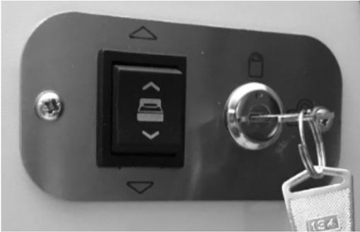
If fitted to your motorhome, the bed control panel will be positioned next to the main control panel located above the habitation entrance door.
