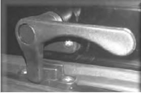
The retaining catches are as previously described on side window catches and can also be positioned to night vent.
