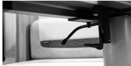
Turn the lever (below the table top) to the right in order to lock the table at its preferred height. If you wish to lower the table, pull the lever 180° so that it is to the left. You can then push the table down as the "brake" has been released. As soon as the table is in the lowest position turn the lever 180° again (to the right) in order to fix it in its lowest position.
