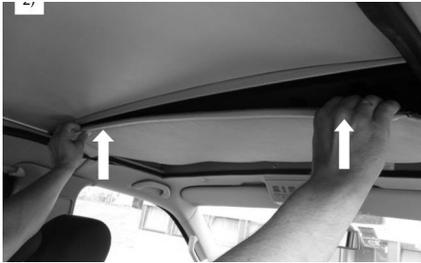
**Note:** Fix the access cover with the press stud fasteners with a certain pretension.
