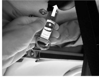
4. Release the locking of the roof according to the following four steps:
