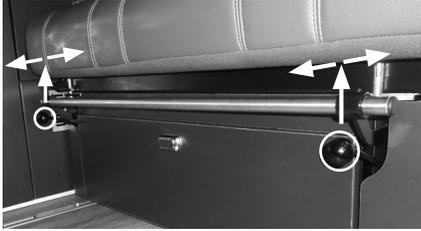
**⚠ WARNING:** The bench seat **MUST BE LOCKED** when driving! Carriage of passengers is permitted only when the bench is locked in the positions intended for this purpose!
