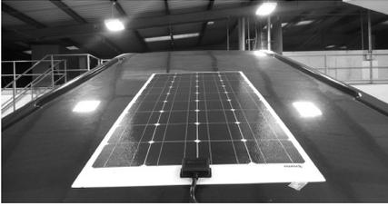
Your campervan is fitted with a solar panel and regulator. This solar panel and regulator may provide additional 12V power whenever sunlight is available to the Camper, and can provide a daily boost to the leisure battery when camping without a mains 230V supply.
