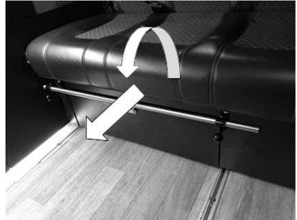
Rotate the front seat base forward revealing the release handle to the right hand side inside the frame.
