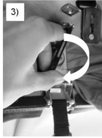
4. Finally, the turning handle is folded upwards.
