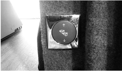
Press one side of the switch to extend the step, the other side to retract the step.
