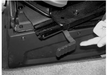
To turn the swivel, slide the BLACK lever rearwards and adjust to the required angle. Before driving off ensure the locking mechanism is fully secure.
