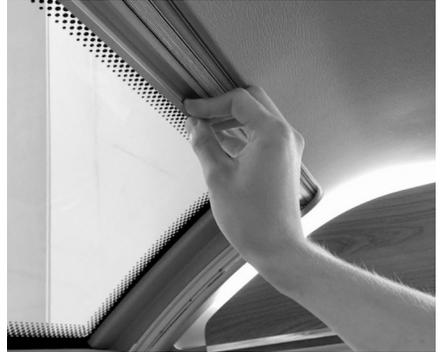
The sunroof blind is operated by pulling the leader rail down. It will then engage into the lower channel. Clean blind with a mild water soapy solution only.
