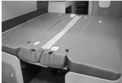
**Step 8:** The back rests are positioned in the middle of the bed. With the backs surface aiming upwards
