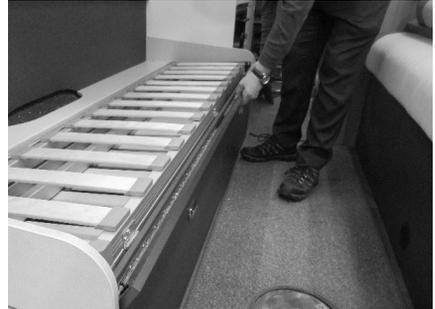
**Step 1:** Remove the Near side bed cushions and release the front facia flap at the top of the bed
