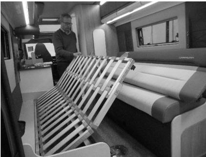
**Step 5:** Moving to the end of the bed lower the extended bed frame over the off side seat base.
