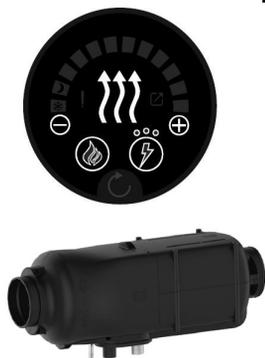
The Whale Heat Air is a dual fuel blown air space heater fitted beneath the motorhome. The controller mounted above the entrance door allows the selection of 230v / mains electric bottled gas energy sources to heat your motorhome, when they are available, along with selection of target room temperature. A 12v fan within the heater distributes heated air through the motorhome via furniture mounted outlets.
